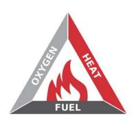
Each element of the Fire Triangle must be in place for combustion to occur. The fire is extinguished when one of the elements is removed from the reaction. The longer this takes the harder it is to suppress the fire as it transforms from a surface fire to a substance fire.
