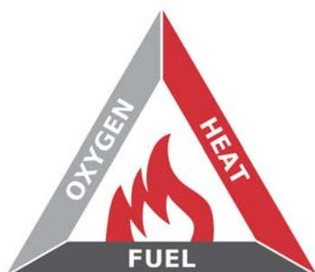
Each element of the Fire Triangle must be in place for combustion to occur. The fire is extinguished when one of the elements is removed from the reaction. The longer this takes the harder it is to suppress the fire as it transforms from a surface fire to a substance fire.
